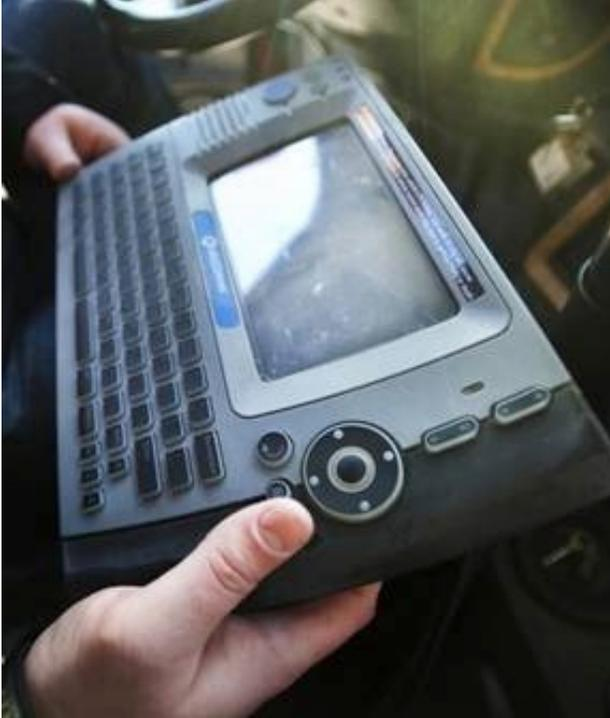
An Electronic On-Board Recorder (EOBR) is an electronic device that connects directly to a vehicle's engine Electronic Control Module (ECM). It records the amount of time the vehicle is being driven, and collects engine diagnostic and GPS data to help fleets optimize operations and automate regulatory compliance.
